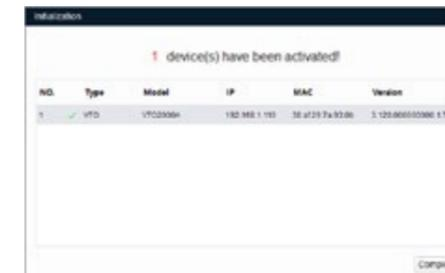
6. The VTO will now show in the Config Tool in an initialised state. It is now possible to program the VTO IP address and other settings.
