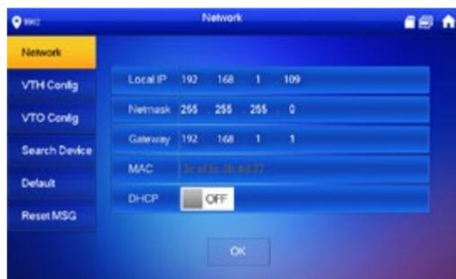
For both the VTO and VTH to communicate, each unit must have the IP address details of the other unit. To add the VTO unit to the VTH, select **VTO Config** and input the VTO units IP address and set **Enable Status** to **ON**.
