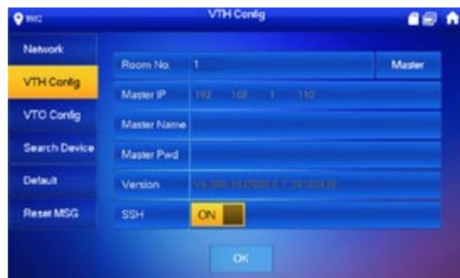
In the settings menu select **Network** to configure the VTH network settings. When configuring the network address of the VTH it is vital to ensure the IP address range is within the same Subnet as the VTO.
