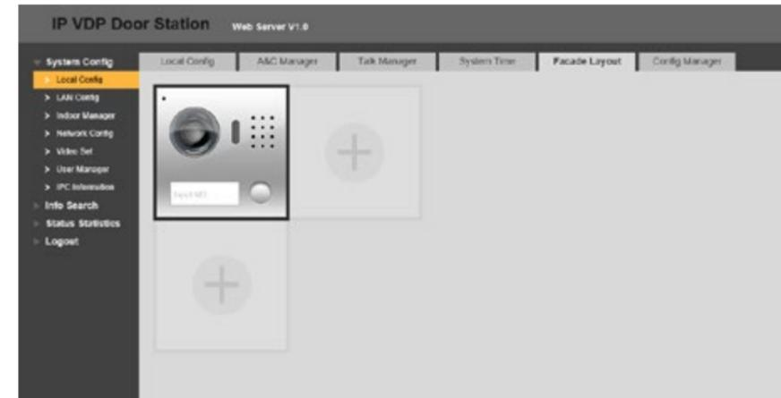
Click the **Plus** symbol in the location of the next module, then select the module type. Multiple modules can be added to the layout.
