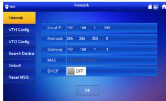
For both the VTO and VTH to communicate, each unit must have the IP address details of the other unit. To add the VTO unit to the VTH, select **VTO Config** and input the VTO units IP address, Username & Password then set **Enable Status** to **ON**.
