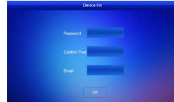
To configure the VTH unit use the built in menu within the monitor itself. VTH units do not support web browser configuration.
