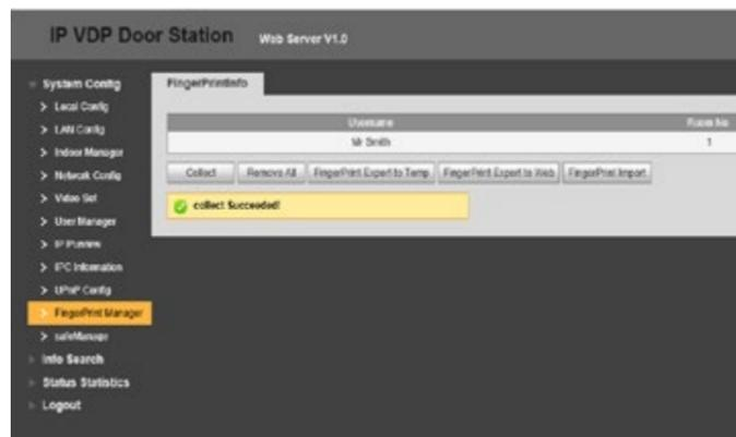
All fingerprints will be displayed in the Fingerprint Manager along with each username. From here, fingerprints can be erased or modified.
