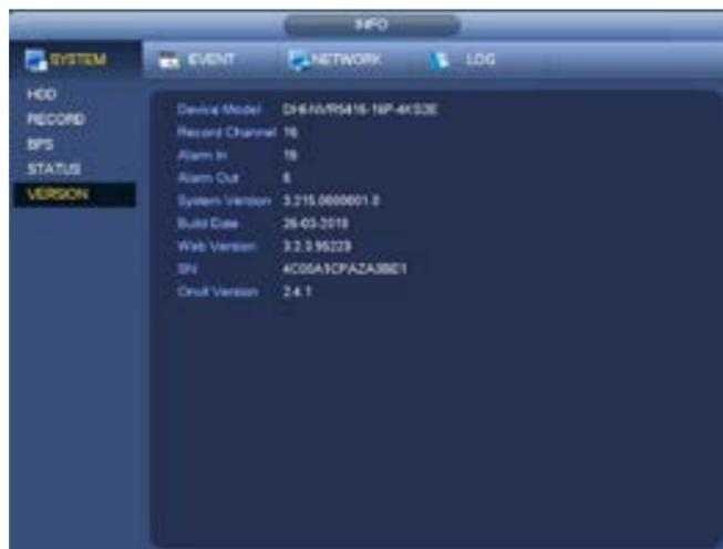
NVR/DVR firmware is often updated to introduce better optimisation and add new features. To check the firmware currently installed on the system go to **Menu > System Info > Version**
