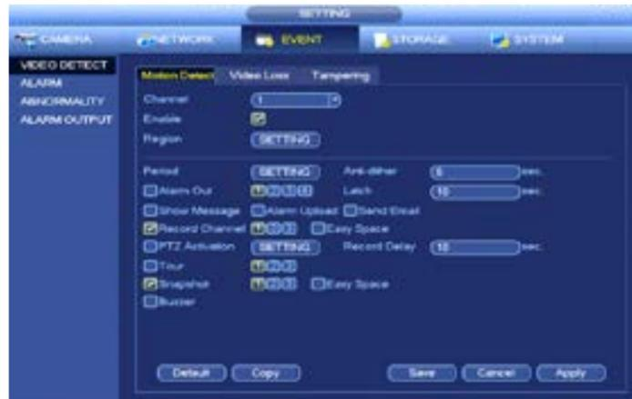
To enable motion detection select the **Enable** box.
