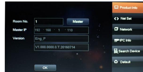
Select **Settings** and then **Project Settings**, in the project settings menu select **NetSet** to configure the VTH network settings. When configuring the network address of the VTH it is vital to ensure the IP address range is within the same Subnet as the VTO.
