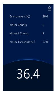
To take a temperature, place your wrist 1cm -4cm to the temperature measurement module. The screen displays as follows.
