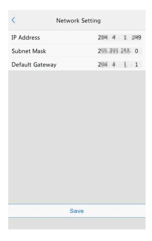
Set the network parameters by referring to the table below. Then tap save to complete network setting.
