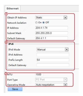
2. Set Obtain IP Address as shown in part 1 of the figure above.
