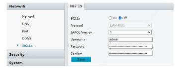
802.1x provides authentication to devices trying to connect to a network. Only the authenticated devices can connect the network. This enhances security.
