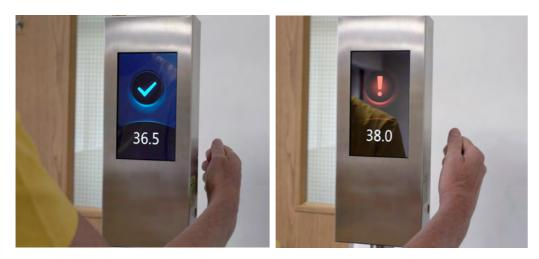
An example of the T-CHECK I unit in operation - The unit offers clear and easy to read indicators of the skin temperature reading.
