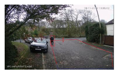
Once the IVS programming has been finished and saved, objects passing through the IVS rule that fit the target filter profile, will trigger and event. This is indicated by the IVS rule flashing red and the configured triggers taking place.
