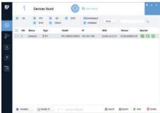
Before adding a camera to a Dahua PoE NVR manually, the IP address of the camera must be programmed to the same range as the Dahua NVR PoE switch. By default Dahua NVR PoE switches are set to **10.1.1.1**
