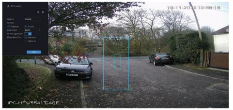
Click the **G** to adjust the target filter. The target filter sets the size of objects that will trigger the IVS rule and the size of objects that will be ignored.
