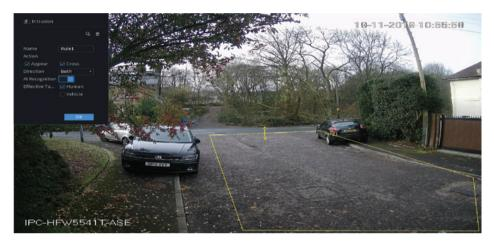
Rules can be created using the left mouse button to draw Tripwire or Intrusion lines on the image in the area of intereset. In the top left window, the direction of travel can also be selected. Once the rule is configured, click **Ok**
